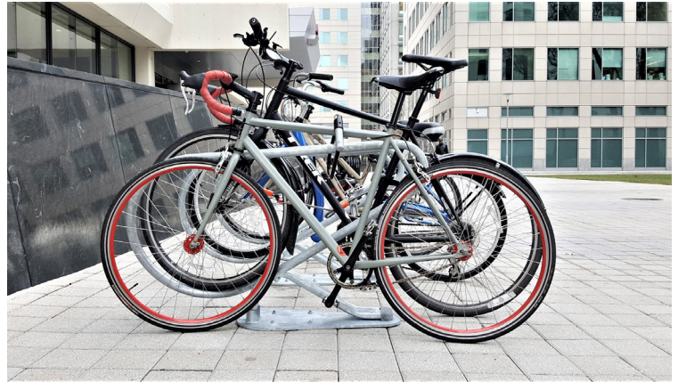
Side view. 400 Tech Square, Cambridge, MA. The longer rack frame and offsetting handlebars makes bikes more stable and less likely to tip over.
